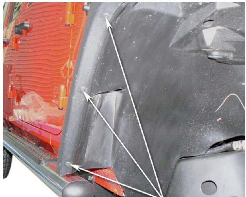
Remove Plastic Pop Rivets
