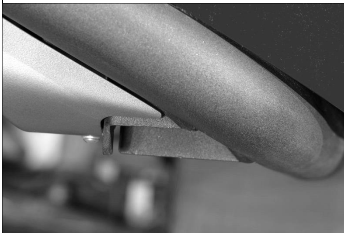
HIGH LIFT JACK LOCATION - CORNER OF RSTB
