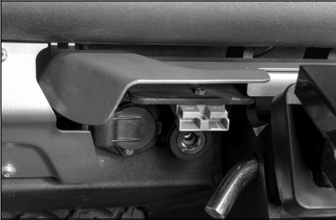
TRAILER CAMERA PLUG, ANDERSON PLUG AND AIR-LINE FITTING
